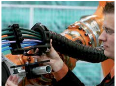
Mounting an igus® triflex® R cable carrier 3D guide on an industrial robot
