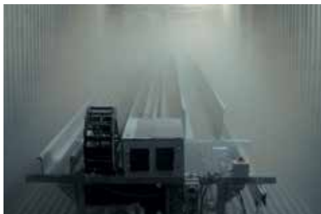
Cold test: chainflex® cables and e-chains® are tested at -40°F (-40°C)
