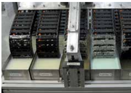
Chemical tests: Testing the effects of a variety of materials on e-chains®
