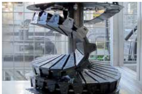
Rotary motion tests: Demanding applications with small radii
