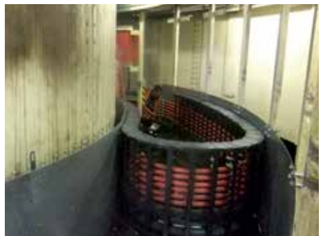
Fully assembled e-chain® with reverse bending radius for circular movement
